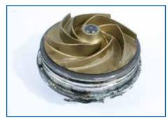
Damage Improper use of sealant
