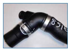
**Damage** Incorrect positioning of the hose clamps
