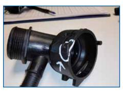
**Damage** Damaged connector
