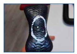
**Damage** Crank in folded area
