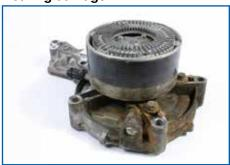
**Damage**Bearing damage due to leakage
