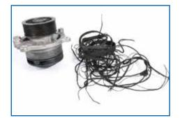
Damage Incorrect belt tension
