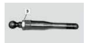
Image 1: The ram of the clutch booster can be adjusted
