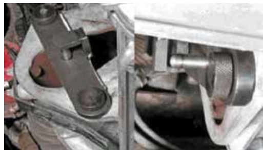
Image 1: The ram of the clutch booster can be adjusted
