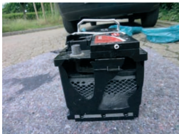
Battery with terminal damage. Clearly visible deposits!
