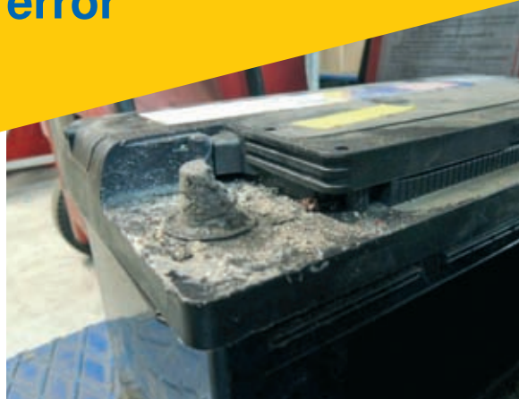
Serious damage: battery casing and grid Possible cause: overloading or wrong charging mode
